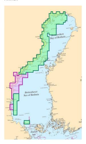
Example of ENC Approach from Sweden: Green cells are referring to the new chart datum BSCD2000, purple cells are ongoing adjustments to BSCD2000 and the rest of the cells refer to various Mean Sea Level.
