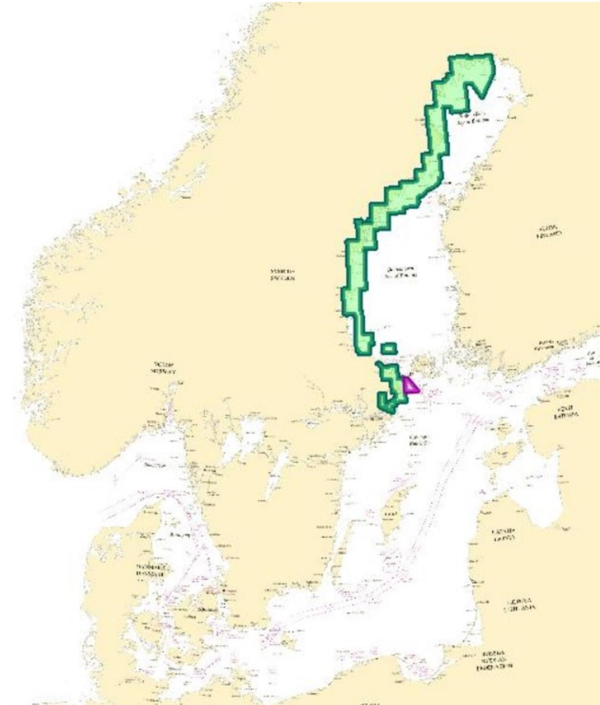
Example of ENC Approach from Sweden (updated 2021-06-21): **Green** cells are referring to the new chart datum BSCD2000, **purple** cells are ongoing adjustments to BSCD2000 and the rest of the cells refer to various Mean Sea Level.
