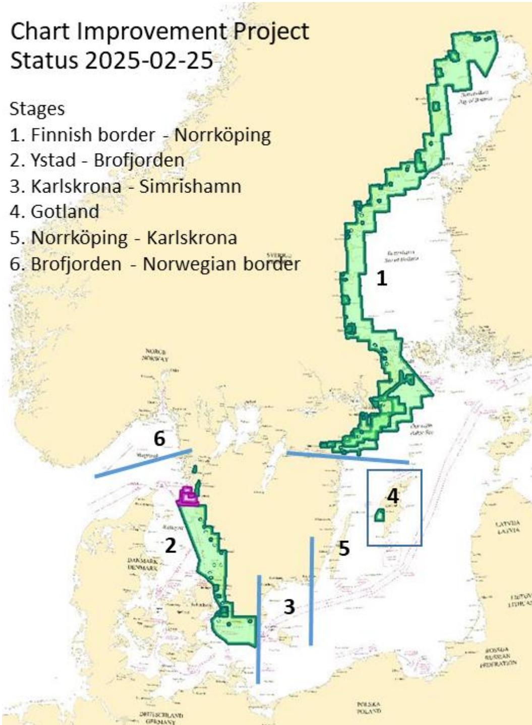
ENC Approach/Berthing from Sweden (updated 2025-02-25): **Green** cells are referring to the new chart datum BSCD2000, **purple** cells are ongoing adjustments to BSCD2000 and the rest of the cells refer to various Mean Sea Level.
