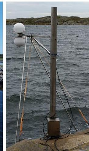
An upward- and downward looking GNSS-reflectometer.
